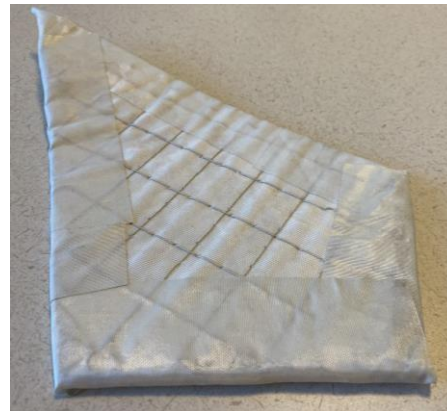
Quilted laser cut material wrapped around the edges
